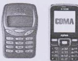
These are basically Time division multiple access (TDMA) or Code division multiple access (CDMA). TDMA allows division of signal into time slots. For communication over a multiplex physical channel CDMA allocates each user a special code. Some of TDMA technologies are GSM, PDC, iDEN, IS-136. Examples of CDMA technology is IS-95. The most admired standard of all the mobile technologies is GSM (Global system for mobile communication).
